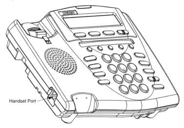
Figure 2-2 Plugging Handset Cord into Telephone
